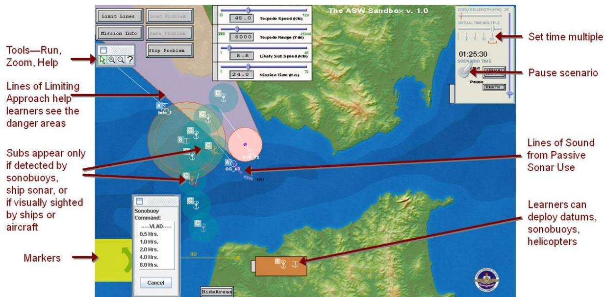
**Figure 1:** Snapshot of the TAO Sandbox user interface, which can be used by instructors to create simulated ASW scenarios involving the deployment and control of helicopters, sonobuoys, ships, and sonar systems. Trainee solutions provided are recorded for later review by instructors.
