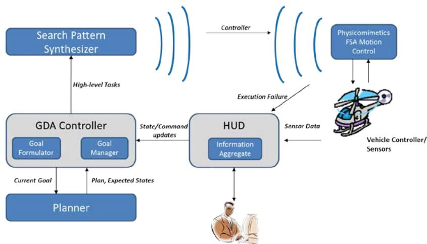
Figure 3. The GDA architecture for controlling the UAVs.
